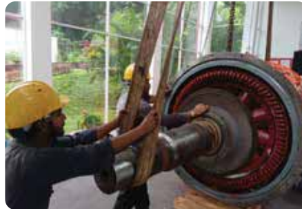
In-house repair work carried out our team at Kiriwaneliya MHP
