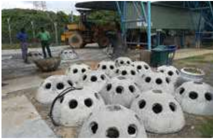
Ready Mix Concrete samples discarded in the quality testing process are upcycled to make the Reef Balls used for coral replanting
